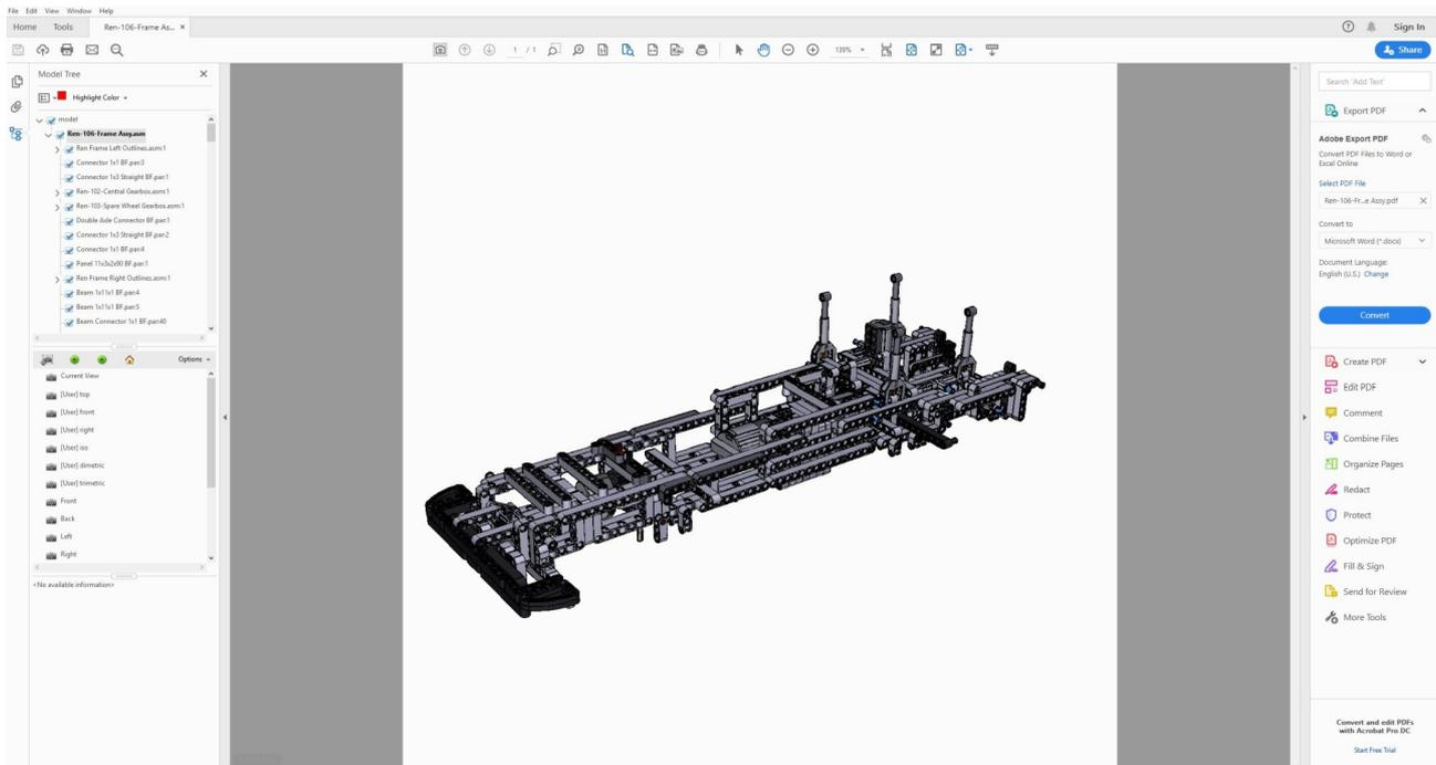
Here you see sub-assemblies and parts together in the REN-106-Frame Assembly. The sub-assemblies you have build before, so you don't have to see their parts now. To prevent the computer from getting slow, there are a great number of parts removed from the sub-assemblies before placing them here and you see the text *Outlines* behind the name now.
