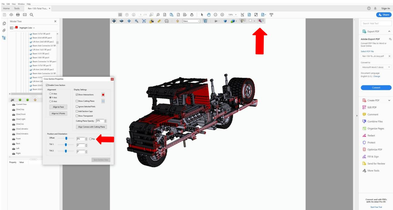
And you can also make section views (top arrow) and by moving this slider (arrow below left) you can slice through the model where you want it in the x, y, or z direction. Here it is the Y-Axis, see in the window.
