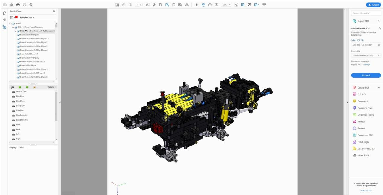
Then you see sub-assemblies and parts together in this SKG-113-Front Frame Assy. The sub-assemblies you have build before, so you don't have to see their parts now (here the SKG-Wheel Set Front Outlines). To prevent the computer from getting slow, there are a great number of parts removed from the sub-assemblies before placing them here and you see the text *Outlines* behind the name now.
