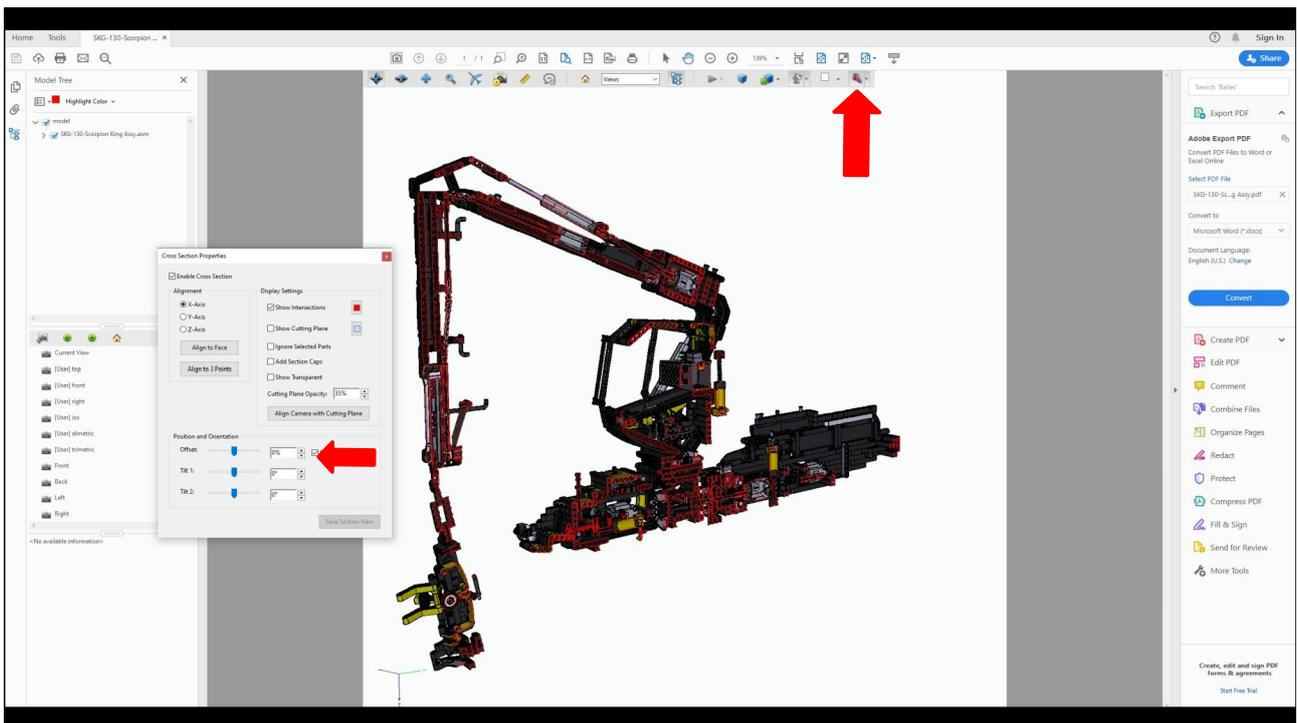
And you can also make section views (top arrow) and by moving this slider (arrow below left) you can slice through the model where you want it in the x, y, or z direction. Here it is the Y-Axis, see in the window.
