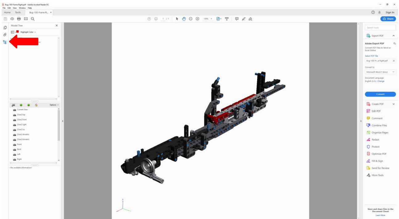
Click here to open the Model Tree. The Model Tree shows a list of all parts and sub-assemblies in the building sequence.
