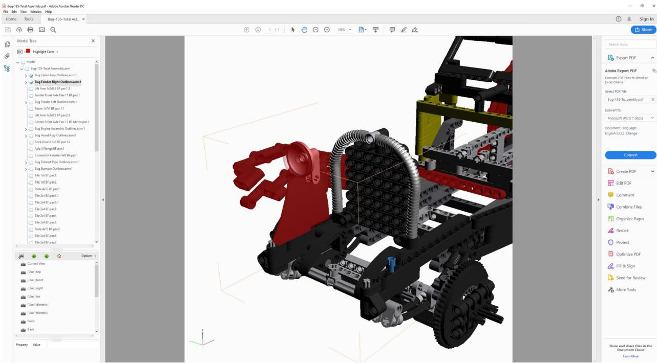
Removing parts from the sub-assemblies makes it also more clear how to place the next parts: here you see the placement of the Right Fender for example.
